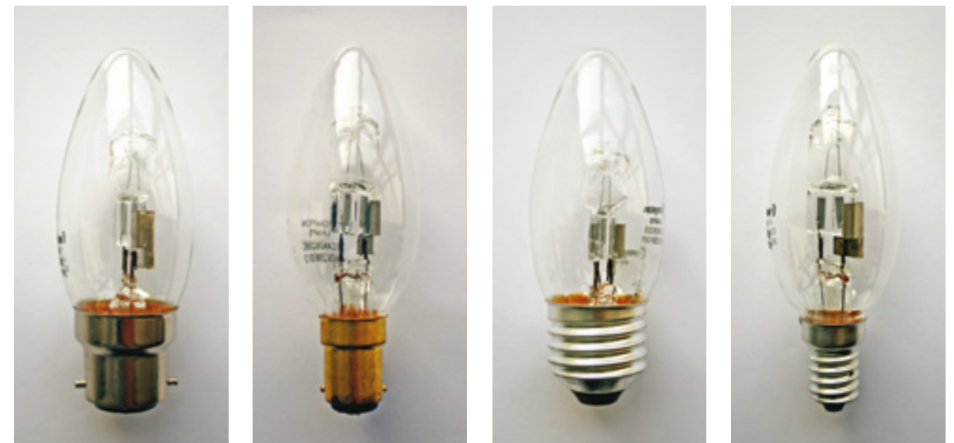
Above, from left: Standard sized bayonet fitting (BC/B22); Small bayonet fitting (BS/B15); Standard screw fitting (ES/E27); Small screw fitting (SES/E14)
